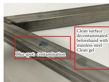
After a reaction time of 30 - 60 seconds, a deep blue spot will appear if ferrite contaminations are present on the surface
