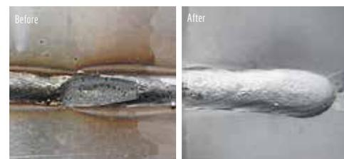
Weld treatment before and after with KPTNOX<sup>18</sup>
